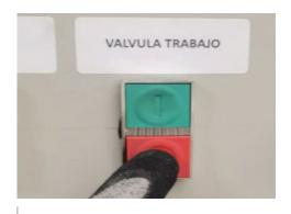
Push the work valve off button
