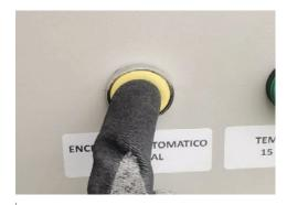
Press the automatic ignition button for 5 seconds
