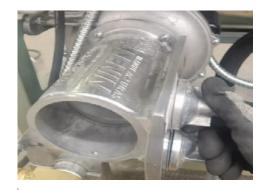
Turn the upper carburetor valve knob to adjust the air intake
