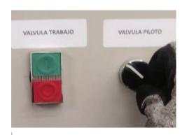
Turn the pilot valve knob, and indicator and the burners will turn off
