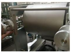
Adjust the tortilla thickness by turning the adjustment knobs (clockwise to make the tortilla thinner, and counterclockwise to make it thicker) Lower the clutch lever when you obtain the desired thickness
