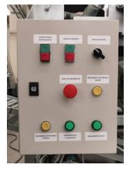
At the end of the day's production it is important to turn off the WORKING VALVE first, then turn off the oven motors second, once the griddles have cooled
