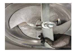
Rotate the assembled auger counterclockwise.
