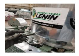
3 Disassemble cross bar rod rod and remove.
