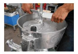
Remove auger of the hopper.
