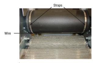
At the end of the day, carefully clean the rollers, especially the straps and the wire, trying not to leave dough residues that could cause the wire to break the next time it is used.
