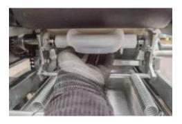
Place the cutter on the base, and verify that it is correctly installed and secured.
