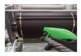
Spray grooves and straps with water **15** to remove excess product.
