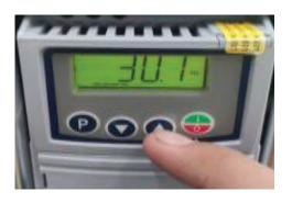
Adjustment of griddles rotation speed at 24 Hz (buttons with arrows, decrease, and increase)
