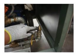
Connect gas hose to the carburetion system (factory carbureted equipment)
