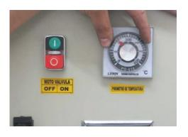
Rotate temperature pyrometer to 180° (dry product) or 220° (wet product)
