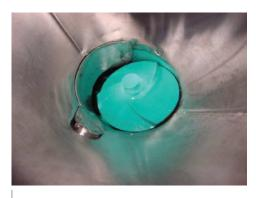
When the lever is pulled up, the tab rises allowing the circulation of corn.
