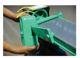
Before moving the lever, secure the counterweight by turning it and inserting the bolt into the desired hole.
