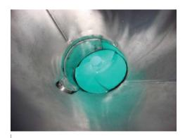
By directing the lever downwards, the tab closes, preventing the circulation of corn.
