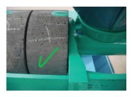
Verify the correct assembly of the stone in the cone plate.
