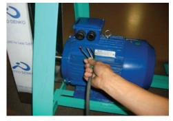
Connect to a 220v two or three phase outlet as the case may be, following the diagram on the plate or on the reverse of the motor cover.
