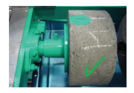
Verify the correct assembly of the stone in the auger plate.
