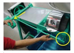
Use the counterweighted lever to adjust the drilled sills into the cone side pins on both sides.
