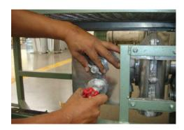
Check that the carburetor tap is at 0 and open the gas stopcock to the carburetor valve.
