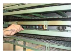
Light the burners with a lighter and start carburizing until the desired flame is obtained.
