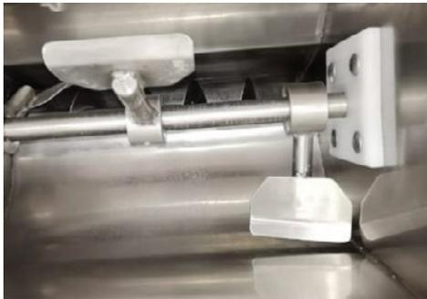
**3** | Before turning on the extruder, check that it is clean and without dough residue.
