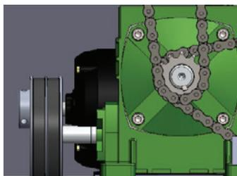
It is recommended to change the oil every three months. The used oil must be drained and 400 ml of new SAE 80/90 oil must be poured.
