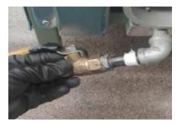
Connect stopcock to carburettor valve inlet.
