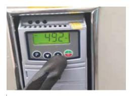
Modify the working speed of the metal bands by 6 pressing the speed drive buttons.
