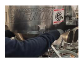
Turn the bolts counterclockwise and remove the hopper.
