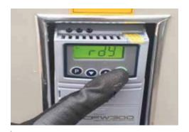
Press the ON (green) button of the speed drive.
