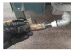
Connect stopcock to carburettor valve inlet.
