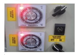
When the press reaches temperature the pyrometer indicator (OFF) will turn on
