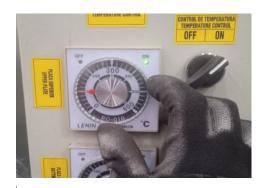
Rotate upper plate pyrometer. The green (ON) indicator will light
