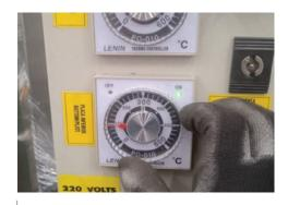
Rotate bottom plate pyrometer. The green (ON) indicator will light
