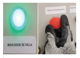
In case of failure, the indicator will illuminate. Extinguish the flame by pressing the emergency stop button
