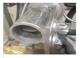
Turn the lower carburetor valve knob to adjust the gas input
