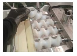
Extract the augers by turning the central ones clockwise and the lateral ones counterclockwise.
