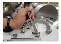
Adjust the thickness of the tortilla with the ratchet
