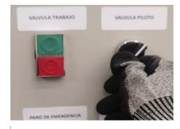
Turn the pilot valve knob, the indicator will illuminate
