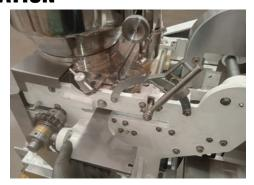
Insert cutter into the head unit
