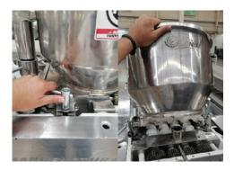
Loosen frame knob and remove the hopper from the head.
