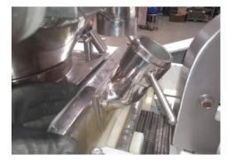
Lower coupling and extract pressure chamber
