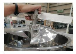
Remove assembled auger by turning counterclockwise and pulling up
