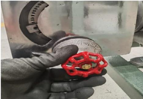
**9** Regulate valve air with a globe key to control the combustion of the machine.
