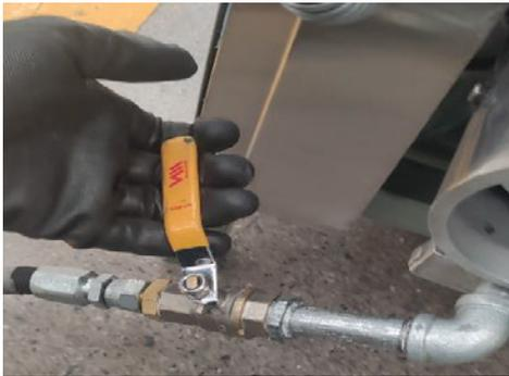
**7** Connect the stopcock to the carburettor valve.
