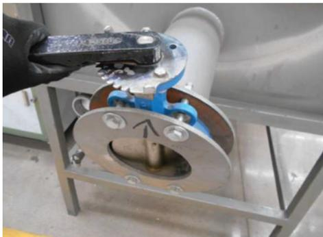
**1** Before introducing the product in the cooker, check that the flood gate is completely closed.
