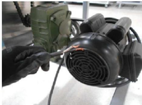
**2** Connect cables from the carburetor valve and motor to a 220v power outlet (two-phase or three-phase, as the case may be).
