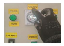
Turn pyrometer to 100°C. "Equipment in operation" indicators will light.
