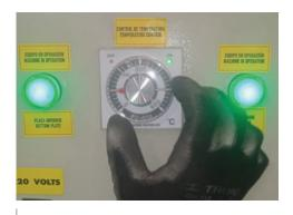
Turn pyrometer to 140-160°C. "Equipment in operation" indicators will light.
