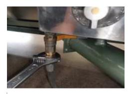
Connect gas outlet to inlet 6 of the carburetor valve.
