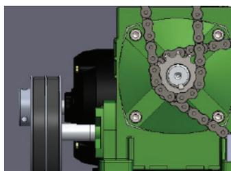
It is recommended to change the oil every three months. The used oil must be drained and 400 ml of new SAE 250 or 80/90 mineral oil must be added.
