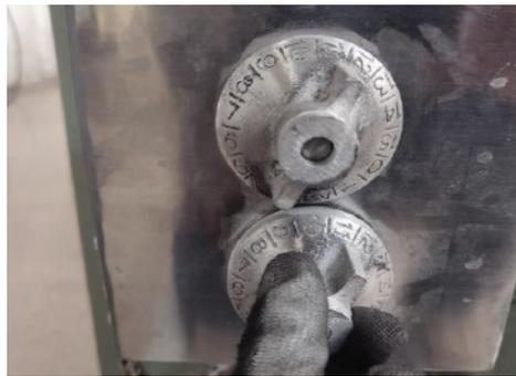
**16** Turn the lower knob of the carburetor valve to regulate the intensity of the flame.
