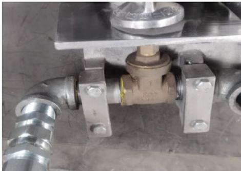
**13** Connect gas outlet to carburetor valve.
