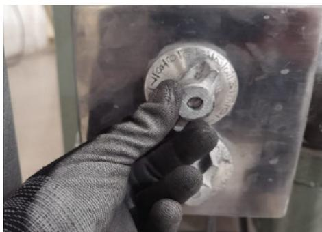
**17** Turn the upper knob of the carburetor valve to regulate air
