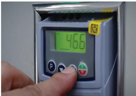
**9** Increase main motor speed by pressing the up arrow button.
