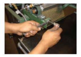
Adjust tortilla thickness at bottom by turning knobs only if necessary.
