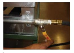
Verify that the griddle and press knobs are well closed. Proceed to open the gas stopcock.
