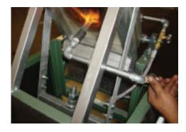
Light the lower plate burner and regulate the flame with the knob.
