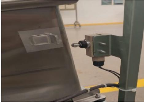
**13** As the hopper does not have contact with the microswitch the mixer will turn off.
