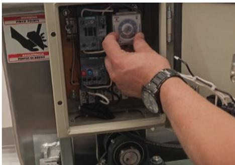
**5** Turn the timer knob adjusting from 0 to 10 minutes.
