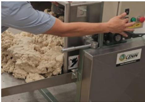
**15** If the motor button is activated, the mixer will not work until it contacts the microswitch
