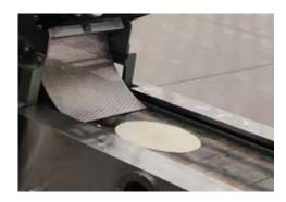
19 Check the shape and thickness of the tortilla.
