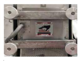
Tortilla thickness adjustment by turning the knobs:
